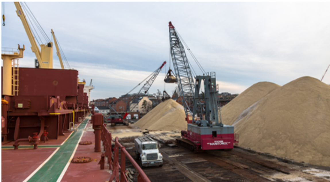
Figure 3: A pair of Manitowac mobile cranes move the salt cargos from ship to shore.
