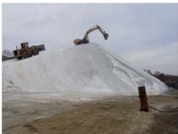
④ Once the salt is moved into the stockpile areas, loaders and dozers shape the pile to be covered.
