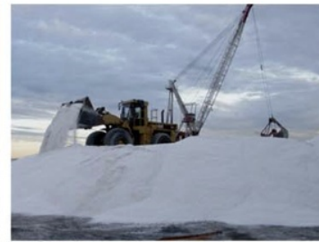
③ Front-end loaders build the pile.
